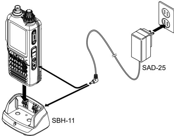
You may insert the cable plug of the **SAD-25** into the **EXT DC** jack located on the right side of the transceiver directly. In this case, the “
