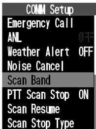
4. Select the desired scan operation by pressing the [▲] or [▼] key, and then press the [ENT] key.
