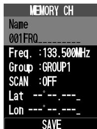
3. After all the inputs or changes have been done, press the [SAVE] key, or select "SAVE" at the bottom of the display with the [▲] or [▼] key, then press the [ENT] key to store them into the memory.
