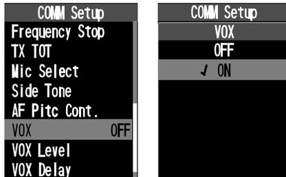
The “**V**” icon, which indicates that the VOX system is active, will appear at the right side of the channel frequency when the display returns to the COM band screen.
