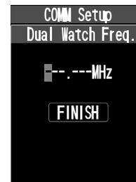
5. Select “**FINISH**” on the screen by pressing the [▲] or [▼] key, and then press the [ENT] key.
