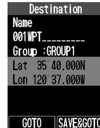
6. Press the [▲] / [▼] keys to select “**GOTO**” and press the [ENT] key.
