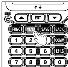
2. Select “**SETUP**” on the MENU screen by pressing the **[▲]** or **[▼]** key, and then press the **[ENT]** key.
