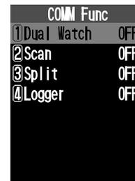
2. Select “**Dual Watch**” on the screen by pressing the [▲] or [▼] key, and then press the [ENT] key.
