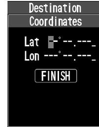
To correct a typo, press the [▲] or [▼] key to move the cursor to the digit to change, and then repeat step 3.
