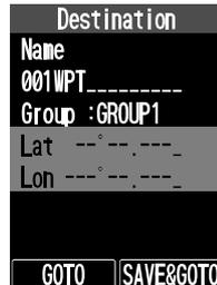
3. Press the keypad or select a number or letter with the DIAL knob and press the [ENT] key.
