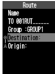
6. Press the [▲] / [▼] keys to select the group in which the desired memory is saved, and then press the [ENT] key.
