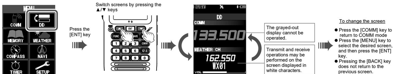
Press the [ENT] key to switch the screen modes that can be operated.
