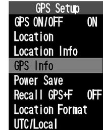
The latitude and longitude of your current position, a radar scope showing the position of captured GPS satellites, bars indicating the signal strength of captured GPS satellites, and the date will be displayed.
