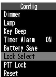
4. Select one of the following lock configuration by pressing the [▲] or [▼] key, and then press the [ENT] key.
