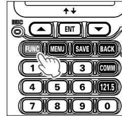
You can also select a function with the **[▲]** / **[▼]** keys or the **DIAL** knob, and then press the **[ENT]** key. Features that are currently unavailable are grayed out.
