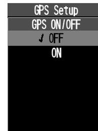
The **"GPS"** icon will appear on the top of the display when returning to the screen of the COMM, MR, or other operation mode.
