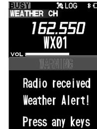
You may enable or disable the alarm function when receiving the weather alert signal via the COMM Setup menu, if desired. See page 76 for details.
