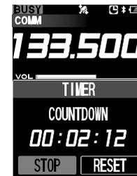
8. To clear the count, select “RESET” on the screen by pressing the [▲] or [▼] key, and then press the [ENT] key.
