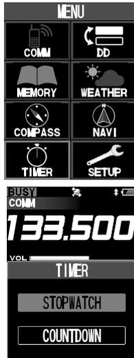
4. To start the counting, select “START” on the screen by pressing the [▲] or [▼] key, and then press the [ENT] key.
