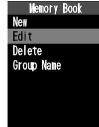
4. Press the [▲] / [▼] keys to select the memory group in which the route you want to edit is saved, and press the [ENT] key.
