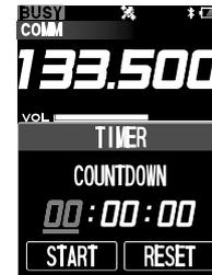
6. To start the counting, select “**START**” on the screen by pressing the [**▲**] or [**▼**] key, and then press the [**ENT**] key.
