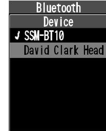
2. Press the [ENT] key. The connection will start. When pairing is complete, “Connected” is displayed.
