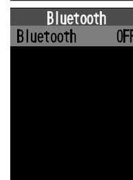
5. Select “ON” on the screen by pressing the [▲] or [▼] key, and then press the [ENT] key.
