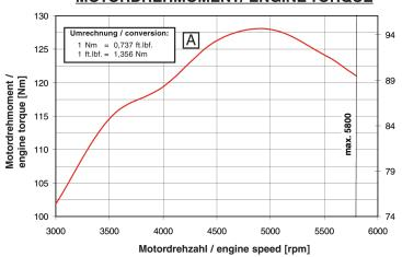
Motordrehmoment / engine torque [ft.lb.]
